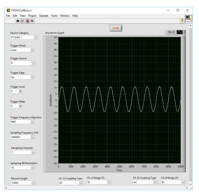
vtDAQCallBack.vi is a sample VI for Labview programming using vtDAQ interfaces. VtDAQ interface wrapper: vtDAQLV.dll, is called using Labview Call Library function node. It is basically an oscilloscope VI with adjustable sampling and triggering parameters. To keep the VI simple, these parameters cannot be changed on-the-fly.
